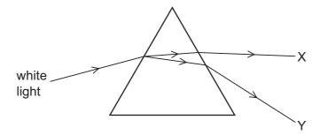
X and Y are the two ends of the visible spectrum.
