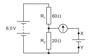
The circuit is to be used to test whether the electromotive force (e.m.f.) of a particular cell is 1.5 V. The cell is connected between terminals X and Y in parallel with R<sub>2</sub> and in series with a galvanometer.
