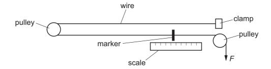
The wire passes from a clamp, around a frictionless pulley, and then to a second frictionless pulley where loads F are applied to it. A marker is attached to the wire so that the total length of wire between the clamp and the marker is initially 3.70 m. A scale is fixed near to this marker.
