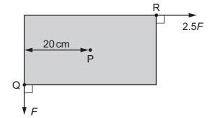
Two forces act in the plane of the board. Force F acts at corner Q and force 2.5F acts at corner R. The perpendicular distance between the line of action of force F and point P is 20 cm. The board is in equilibrium.
