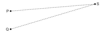
At the point S there is a minimum in the interference pattern produced by waves from the two sources. The distance (QS - PS) is called the path difference.
