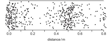
23 When a guitar string is plucked, it causes a longitudinal sound wave in the air, as shown.
