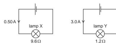
What is the ratio  $\frac{\text{power in lamp X}}{\text{power in lamp Y}}$ ?
