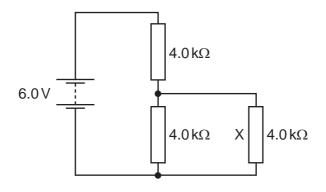
Each resistor has a resistance of  $4.0 \,\mathrm{k}\Omega$ .
