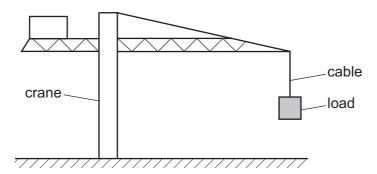
A model is made of the crane, its load and the cable supporting the load.
