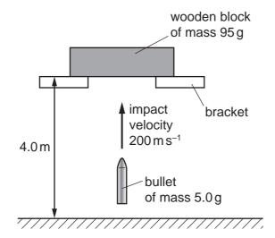
A bullet of mass 5.0g is shot vertically upwards into the wooden block of mass 95g. It embeds itself in the block. The impact causes the block to rise above its supporting brackets.
