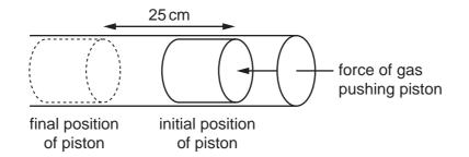
How much work is done by the gas on the piston when it moves through a distance of 25 cm?
