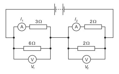
The readings on the meters are  $I_1$ ,  $I_2$ ,  $V_1$  and  $V_2$ , as labelled on the diagram.
