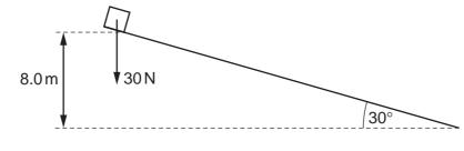
What is the kinetic energy of the box after falling through this distance?
