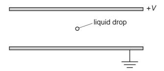
A small charged liquid drop, midway between the plates, is held in equilibrium by the combination of its weight and the electric force acting on it.
