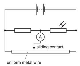
The light-dependent resistor (LDR) is then covered up and the ammeter gives a non-zero reading.
