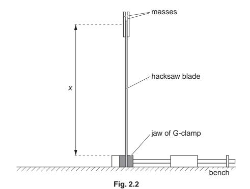
(ii) Measure and record the distance *x* between the top of the jaw of the G-clamp and the centre of the masses, as shown in Fig. 2.2.
