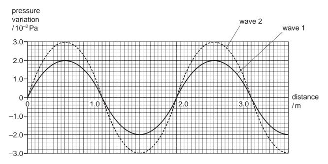
Wave 1 has an intensity of 1.6  $\times$   $10^{-6}\,W\,m^{-2}.$
