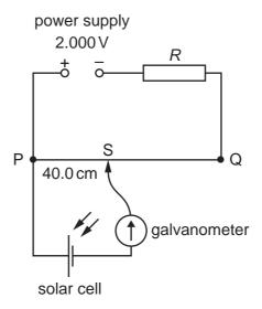
The e.m.f. produced by the solar cell is measured on the potentiometer.
