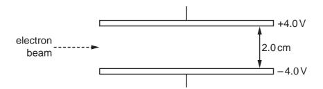
The upper plate has an electrical potential of +4.0 V, and the lower plate has an electrical potential of -4.0 V.
