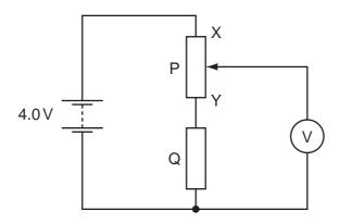
The slider on the potentiometer is moved from X to Y and a graph of voltmeter reading V is plotted against slider position.
