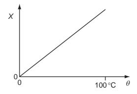
$\theta$  is determined from the corresponding values of X by using this graph. X is measured with a percentage uncertainty of ±1% of its value at all temperatures.
