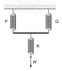
Springs P and Q are identical and have spring constant *k*. Spring R has spring constant 3*k*.
