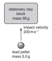
The pellet hits the block with an initial velocity of  $200 \,\mathrm{m \, s^{-1}}$ . It embeds itself in the block and does not emerge.
