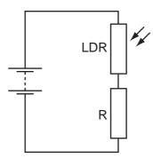
The resistance of the LDR is equal to the resistance of R when no light falls on the LDR.
