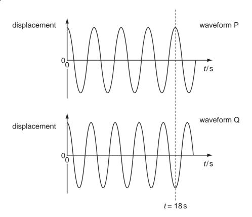
At time t = 0 the waves are in phase. At the dotted line,  $t = 18 \, \text{s}$ .
