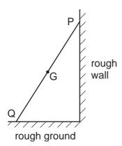
Its weight W acts through the centre of gravity G. Forces also act on the ladder at P and at Q. These forces are P and Q respectively.
