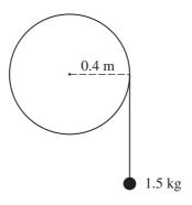
A uniform disc of radius 0.4 m is free to rotate without friction in a vertical plane about a horizontal axis through its centre. The moment of inertia of the disc about the axis is  $0.2 \, \text{kg} \, \text{m}^2$ . One end of a light inextensible string is attached to a point on the rim of the disc and the string is wound round the rim. The other end of the string is attached to a particle of mass 1.5 kg which hangs freely (see diagram). The system is released from rest. Find
