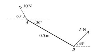
A non-uniform rod AB of length 0.5 m is freely hinged to a fixed point at A. The rod is in equilibrium at an angle of  $30^{\circ}$  with the horizontal with B below the level of A. Equilibrium is maintained by a force of magnitude F N applied at B acting at  $45^{\circ}$  above the horizontal in the vertical plane containing AB. The force exerted by the hinge on the rod has magnitude  $10 \, \text{N}$  and acts at an angle of  $60^{\circ}$  above the horizontal (see diagram).
