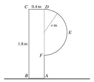
The diagram shows the cross-section ABCDEF through the centre of mass of a uniform prism which rests with AB on rough horizontal ground. ABCD is a rectangle with AB = CD = 0.4 m and BC = AD = 1.8 m. The other part of the cross-section is a semicircle with diameter DF and radius r m.
