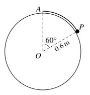
One end of a light inextensible string is attached to the highest point A of a solid fixed sphere with centre O and radius 0.6 m. The other end of the string is attached to a particle P of mass 0.2 kg which rests in contact with the smooth surface of the sphere. The angle  $AOP = 60^{\circ}$  (see diagram). The sphere exerts a contact force of magnitude RN on P and the tension in the string is TN.
