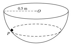
A particle *P* of mass 0.4 kg moves with constant speed in a horizontal circle on the smooth inner surface of a fixed hollow hemisphere with centre *O* and radius 0.5 m (see diagram).
