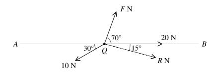
A small bead Q can move freely along a smooth horizontal straight wire AB of length 3 m. Three horizontal forces of magnitudes F N, 10 N and 20 N act on the bead in the directions shown in the diagram. The magnitude of the resultant of the three forces is R N in the direction shown in the diagram.
