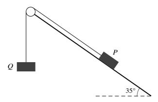
Blocks P and Q, of mass  $m \log a$  and 5 kg respectively, are attached to the ends of a light inextensible string. The string passes over a small smooth pulley which is fixed at the top of a rough plane inclined at 35° to the horizontal. Block P is at rest on the plane and block Q hangs vertically below the pulley (see diagram). The coefficient of friction between block P and the plane is 0.2. Find the set of values of P for which the two blocks remain at rest.
