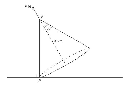
A uniform solid cone with height  $0.8 \,\mathrm{m}$  and semi-vertical angle  $30^{\circ}$  has weight  $20 \,\mathrm{N}$ . The cone rests in equilibrium with a single point P of its base in contact with a rough horizontal surface, and its vertex V vertically above P. Equilibrium is maintained by a force of magnitude F N acting along the axis of symmetry of the cone and applied to V (see diagram).
