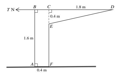
ABCDEF is the cross-section through the centre of mass of a uniform solid prism. ABCF is a rectangle in which AB = CF = 1.6 m, and BC = AF = 0.4 m. CDE is a triangle in which CD = 1.8 m, CE = 0.4 m, and angle  $DCE = 90^{\circ}$ . The prism stands on a rough horizontal surface. A horizontal force of magnitude T N acts at B in the direction CB (see diagram). The prism is in equilibrium.
