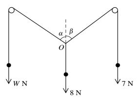
Each of three light inextensible strings has a particle attached to one of its ends. The other ends of the strings are tied together at a point O. Two of the strings pass over fixed smooth pegs and the particles hang freely in equilibrium. The weights of the particles and the angles between the sloping parts of the strings and the vertical are as shown in the diagram. It is given that  $\sin \beta = 0.8$  and  $\cos \beta = 0.6$ .
