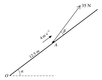
A small block of mass 3 kg is initially at rest at the bottom O of a rough plane inclined at an angle  $\alpha$  to the horizontal, where  $\sin \alpha = 0.6$  and  $\cos \alpha = 0.8$ . A force of magnitude 35 N acts on the block at an angle  $\beta$  above the plane, where  $\sin \beta = 0.28$  and  $\cos \beta = 0.96$ . The block starts to move up a line of greatest slope of the plane and passes through a point A with speed  $4 \text{ m s}^{-1}$ . The distance OA is 12.5 m (see diagram).
