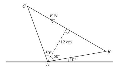
A uniform lamina ABC in the shape of an isosceles triangle has weight 24 N. The perpendicular distance from A to BC is 12 cm. The lamina rests in a vertical plane in equilibrium, with the vertex A in contact with a horizontal surface. Angle  $BAC = 100^{\circ}$  and AB makes an angle of  $10^{\circ}$  with the horizontal. Equilibrium is maintained by a force of magnitude F N acting along BC (see diagram). Show that F = 8.
