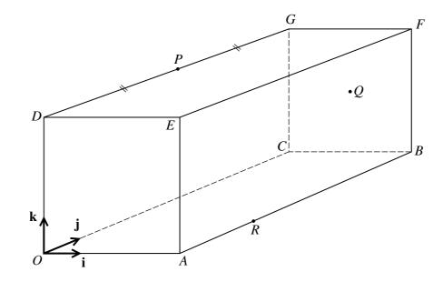
In the diagram, OABCDEFG is a rectangular block in which OA = OD = 6 cm and AB = 12 cm. The unit vectors **i**, **j** and **k** are parallel to  $\overrightarrow{OA}$ ,  $\overrightarrow{OC}$  and  $\overrightarrow{OD}$  respectively. The point *P* is the mid-point of *DG*, *Q* is the centre of the square face *CBFG* and *R* lies on *AB* such that AR = 4 cm.
