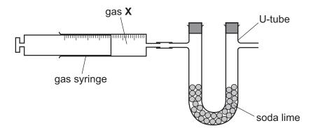
A  $100.0\,\mathrm{cm^3}$  sample of pure gas  $\mathbf{X}$  is placed in a gas syringe. The gas syringe is attached to a U-tube containing small lumps of solid soda lime, a mixture of sodium hydroxide and calcium hydroxide. All of gas  $\mathbf{X}$  is slowly passed into the U-tube and the mass of gas  $\mathbf{X}$  absorbed determined.
