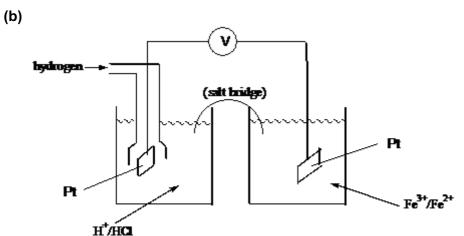
$H_2$  and good delivery system [1]  $Fe^{2^+}/Fe^{3^+}$  solution labelled [1] platinum electrodes (both) [1] salt bridge and voltmeter [1]  $H^+$  or HCl or H<sub>2</sub>SO<sub>4</sub> [1] (acid is not sufficient) [5]
