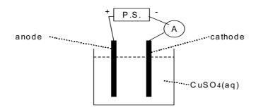
correct cell (2 electrodes + PS circuit) [1] ammeter in series [1] anode and cathode of the right polarity [IN WORDS] [1]
