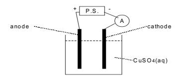
correct cell (2 electrodes + PS circuit) [1] ammeter in series [1] anode and cathode of the right polarity [IN WORDS] [1]
