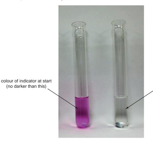
test-tube **E** with indicator showing the colourless end-point
