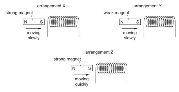
Which arrangement induces the largest electromotive force (e.m.f.) and which arrangement induces the smallest e.m.f.?
