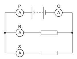
Which two ammeters read the largest current?
