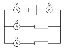
Which two ammeters read the largest current?
