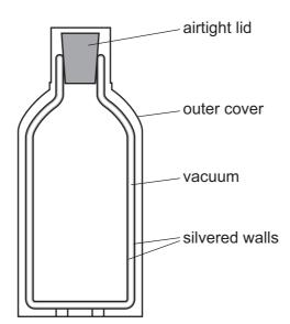
Which methods of heat loss are reduced by the vacuum between the silvered walls?
