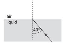
What is the angle of refraction as the light enters the air?
