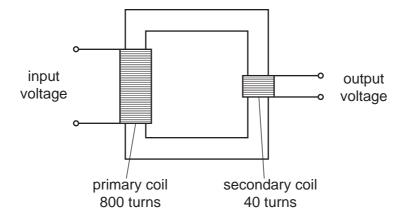
The input voltage is 240 V.
