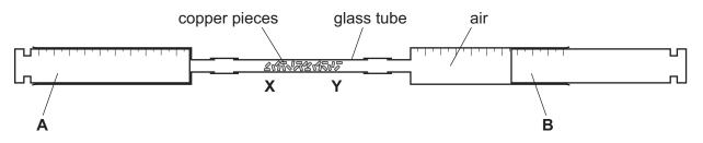
The glass tube was heated strongly at X while the sample of air was passed backwards and forwards over the copper pieces in the tube. The source of heat was gradually moved along the tube from X to Y.
