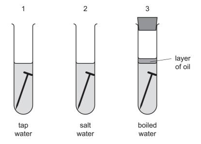
In which test-tubes do the nails rust?
