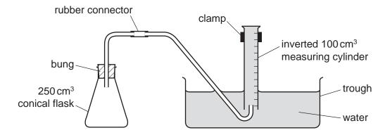
The trough should be large enough to allow the measuring cylinder to be filled with water in the trough.
