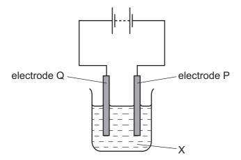
During the electrolysis, sodium was formed at electrode P and chlorine at electrode Q.
