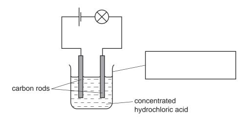
During the experiment, bubbles were observed at both carbon rods.
