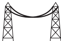
iron cored aluminium electricity cables
