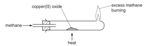
The solid changed colour to red-brown and drops of liquid condensed in the cold part of the tube.
