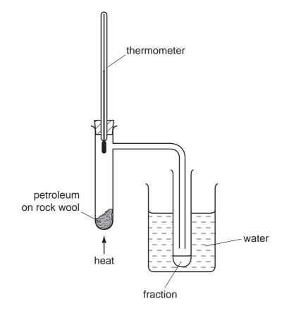
Which fraction contains the smallest hydrocarbon molecules?
