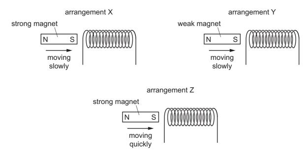
Which arrangement induces the largest electromotive force (e.m.f.) and which arrangement induces the smallest e.m.f.?
