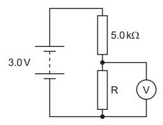
The reading on the voltmeter is 1.8 V.
