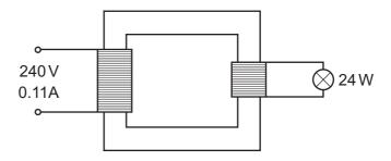
The input current to the transformer is  $0.11\,\mathrm{A}$  and the input voltage is  $240\,\mathrm{V}$ . The useful output power of the transformer is  $24\,\mathrm{W}$ .
