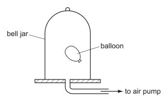
The air pump is switched on and air is removed from the bell jar.
