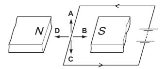
**34** A simple d.c. motor consists of a coil that rotates between the poles of a permanent magnet. The turning effect is increased by winding the coil on a metal cylinder.
