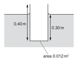
The cross-sectional area of the pipe is 0.012 m<sup>2</sup>. The weight of the pipe is 32 N.
