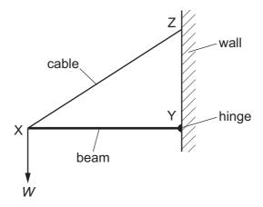
The beam supports a weight W at point X. The forces in the cable and the beam are  $F_C$  and  $F_B$ respectively.
