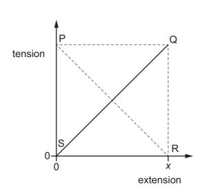
The variation of the tension in the spring with its extension is shown on the graph.
