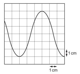
The time-base setting is  $0.5\,\mathrm{ms\,cm^{-1}}$  and the Y-plate sensitivity is  $0.2\,\mathrm{mV\,cm^{-1}}$ .
