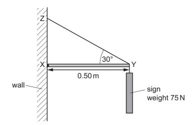
The frame consists of a horizontal rod XY and a rod YZ that is at an angle of 30° to the horizontal. Rod XY is attached to the wall by a hinge at X and has length 0.50 m. Assume that the weights of the rods are negligible.
