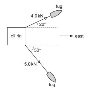
The tensions in the towing cables are 4.0 kN and 5.0 kN.
